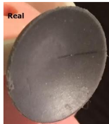
Real Reflector with dark line in smooth plastic
