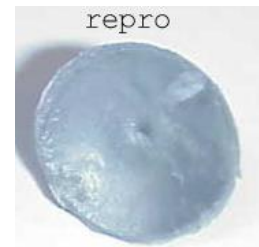
Repro Reflector is rough and uneven and it has no line
